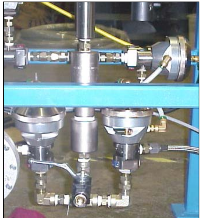
Power Inlet/ Outlet Apollo Valves On High Viscosity, Two Component Metering System
