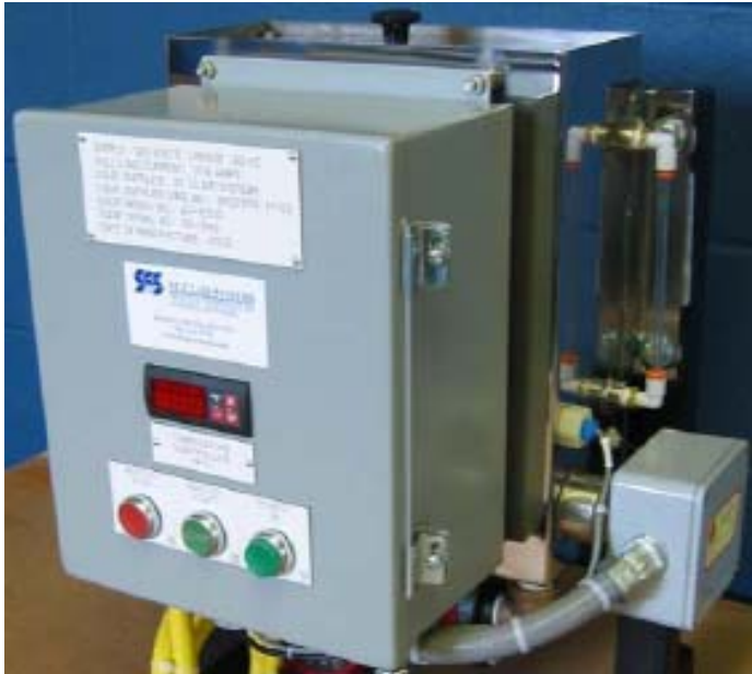
Water Heat-Only Temperature Control System
