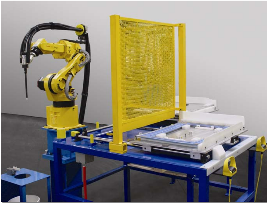
Sealant Equipment & Engineering robotic dispense system dispensing adhesive in a dual station manual transfer fixture
