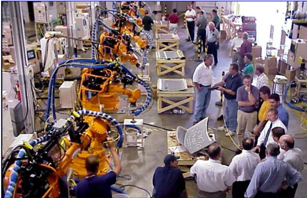
Wet Run-Off for End-User and Automation Line Builder including Cpk Analysis
